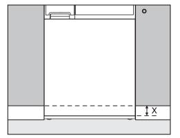
First of all you need to calculate measurement **X**. This is the distance from the lower edge of the machine door to the lower edge of an adjacent kitchen unit door front.
